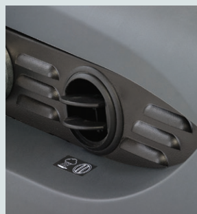
Wet sweep bypass protects the filter from water fouling when sweeping in wet conditions.
